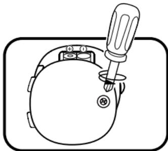
4. Install 2 new AAA (AM-4/LR03) batteries following the diagram inside the battery box. (The use of new alkaline batteries is recommended for maximum performance).
